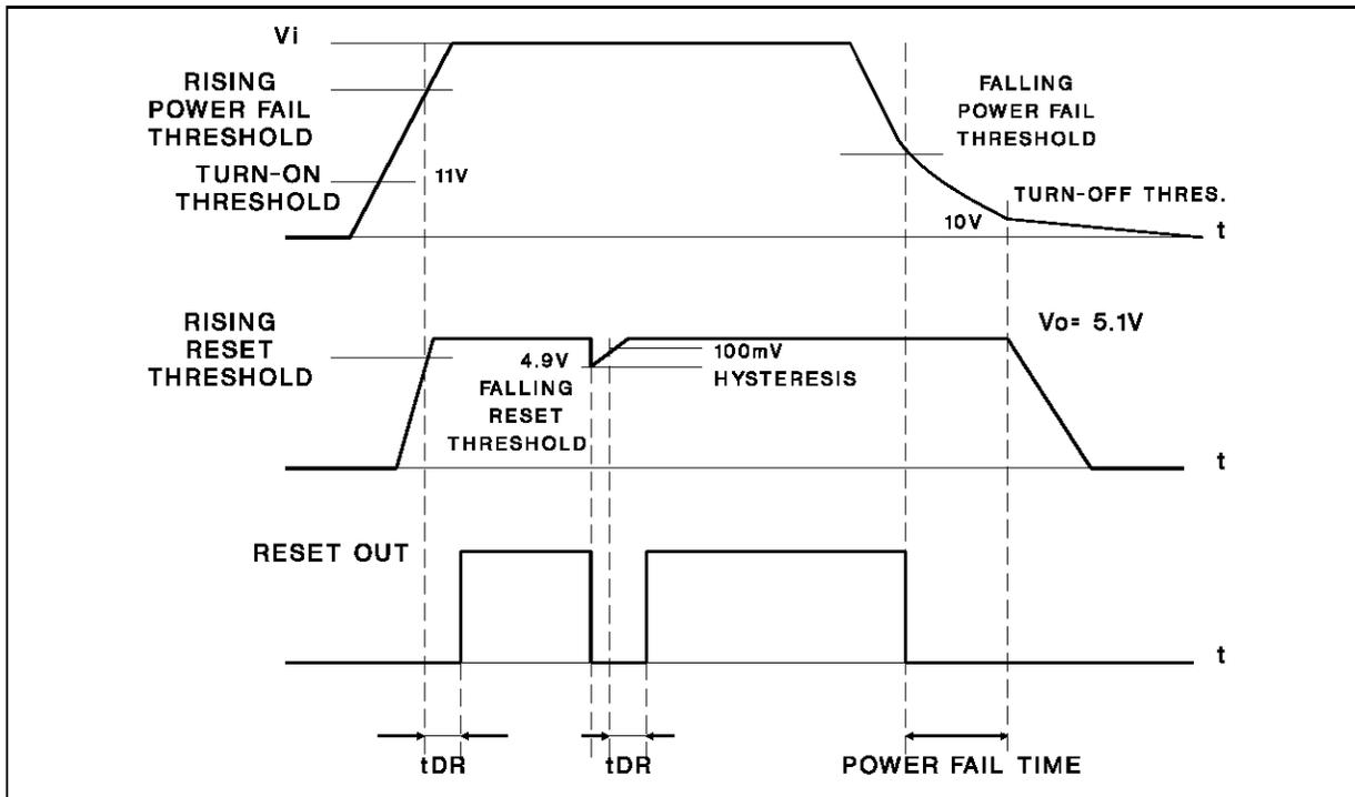
Figure 2 - Reset and Power Fail waveforms.
