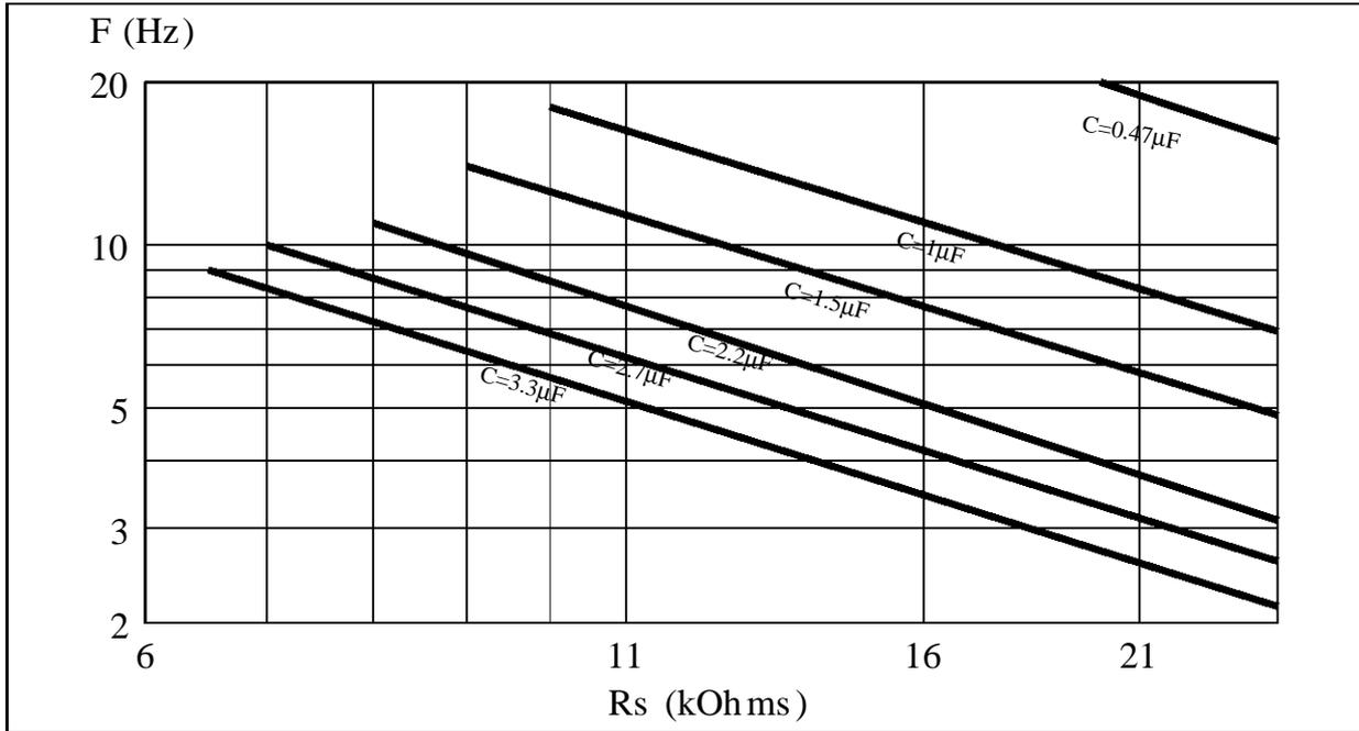
The couple Rs/C can be chosen with the previous curve. Keep in mind the Rs maximum limit for which the system would not work when the AC
