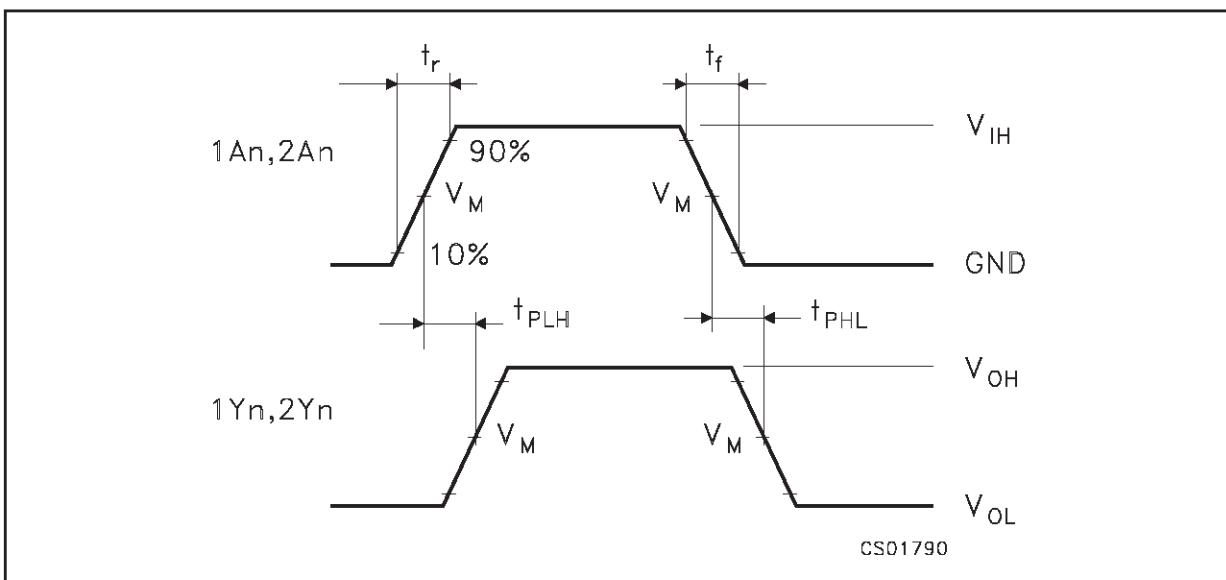
**WAVEFORM 2: OUTPUT ENABLE AND DISABLE TIME (f=1MHz; 50% duty cycle)**
