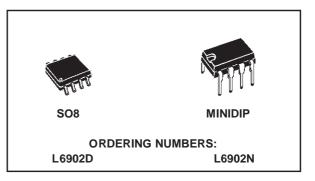
fier to have a constant voltage and constant current control for a most efficient charging solution of the modern rechargeable batteries including lithium-ion, NiMH and NiCd.
