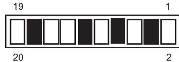
**Note:** Setting the jumper 3-4 causes a verifying operation to be automatically executed after the programming process. This jumper is set in the default configuration (factory setting).
