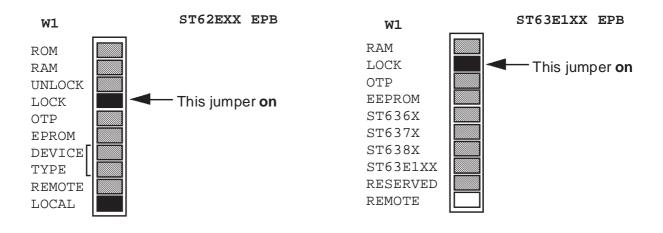
To prevent the device from being ever read-protected, set the UNLOCK jumper. This function is available for devices with the OPTION byte (ST62E2XX only).
