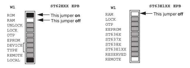
2 Select a reference EPROM, by setting the appropriate jumper combination in the W2 jumper bank:
