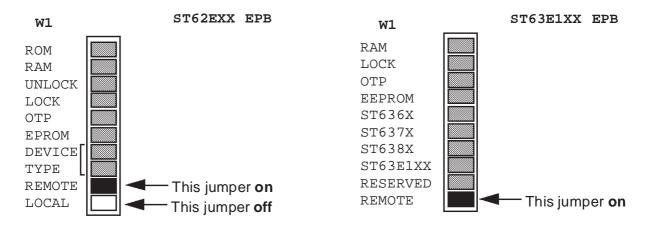
Note: EPBs are shipped with the REMOTE jumper on.
