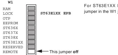
For ST63E1XX EPBs, remove the REMOTE jumper in the W1 jumper bank.
