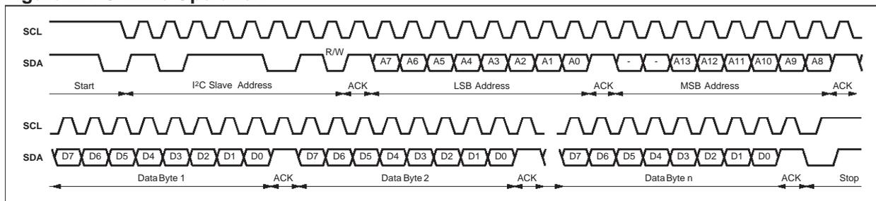
Figure 3. I<sup>2</sup>C Read Operation
