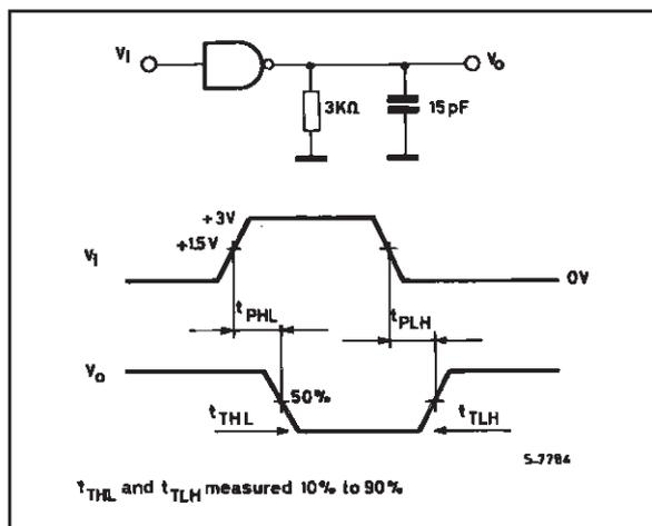
Figure 7 : Transfer Characteristics versus
