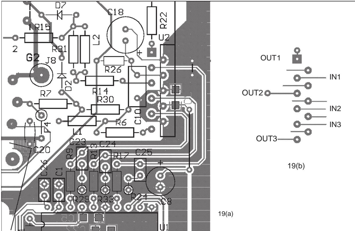
Figure 20. TDA9210 - TDA9535/9536 Demonstration Board Schematic
