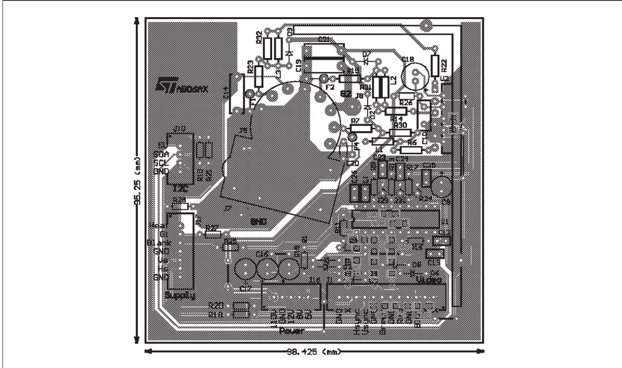
Figure 19. Amplifier and Preamp Output. Trace Routing (detail)
