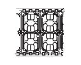
ST currently provides Smartcard ICs in micromodule form in super 35mm tape.
