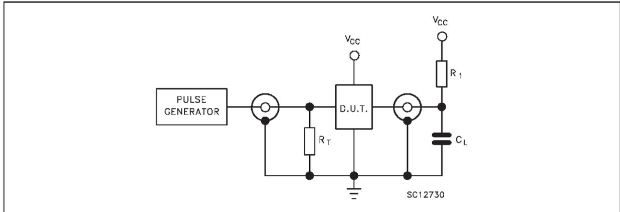
$C_L = 15/50$  pF or equivalent (includes jig and probe capacitance)
