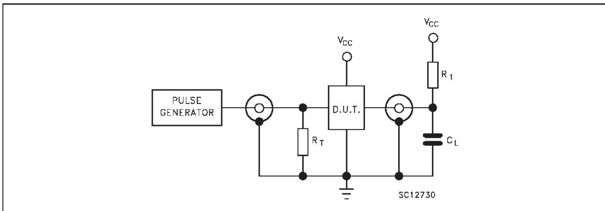
$C_L = 15/50 \text{ pF}$  or equivalent (includes jig and probe capacitance) $R_L = R_1 = 1\text{K}\Omega$  or equivalent $R_T = Z_{out}$  of pulse generator (typically  $50\Omega$ )
