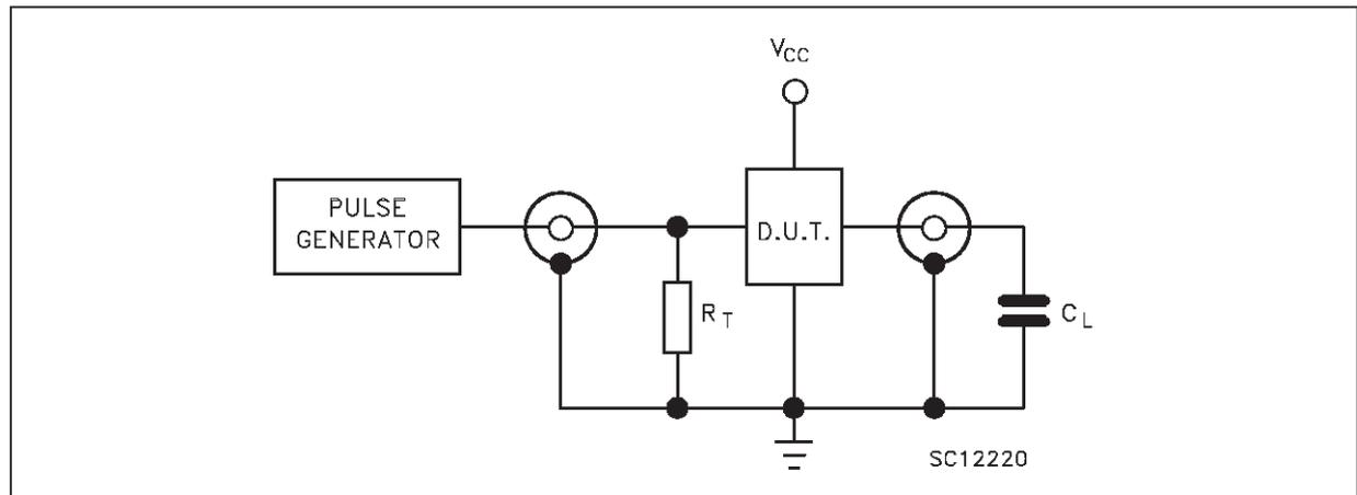
C<sub>L</sub> = 50 pF or equivalent (includes jig and probe capacitance)
