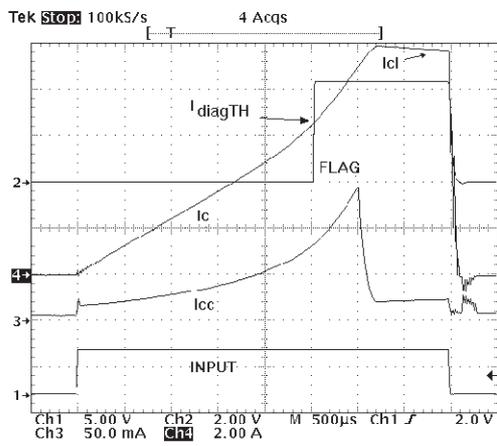
Fig. 2 Output Current Waveform After Thermal Protection Activation
