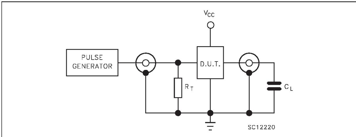
$C_L = 15/50 \text{ pF}$  or equivalent (includes jig and probe capacitance)
