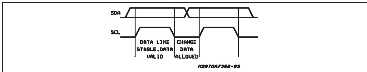
Figure 4. Timing Diagram of I<sup>2</sup>C BUS
