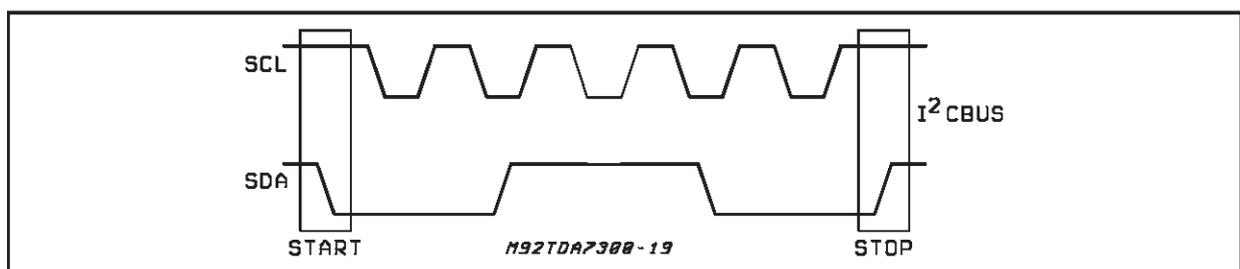
Figure 5. Acknowledge on the I<sup>2</sup>C BUS
