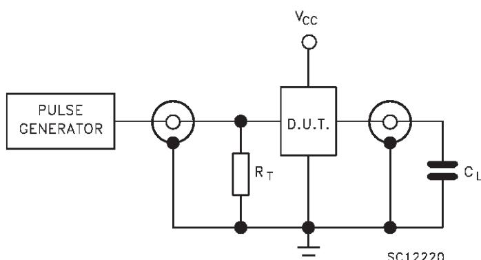
$C_L = 15/50 \text{ pF}$  or equivalent (includes jig and probe capacitance)
