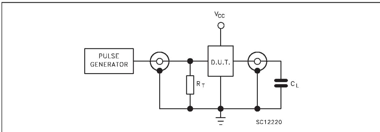
$C_L = 15/50 \text{ pF}$  or equivalent (includes jig and probe capacitance)
