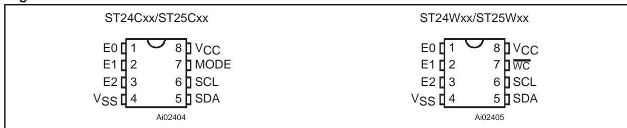
Figure 1. ST24xxx/ST25xxx Pin Connections
