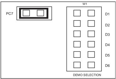
**7** Select the demo you want to run, by installing the appropriate jumper on W1 (marked 2 on the Starter Kit board diagram on page 9), as indicated on the diagram below:
