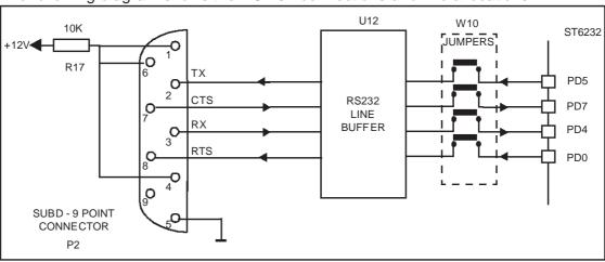
TX, RX, CTS and RTS are defined so that the board is used as a slave. To use the board as a master, swap both the RX and TX and the CTS and RTS pin connections on the cable.
