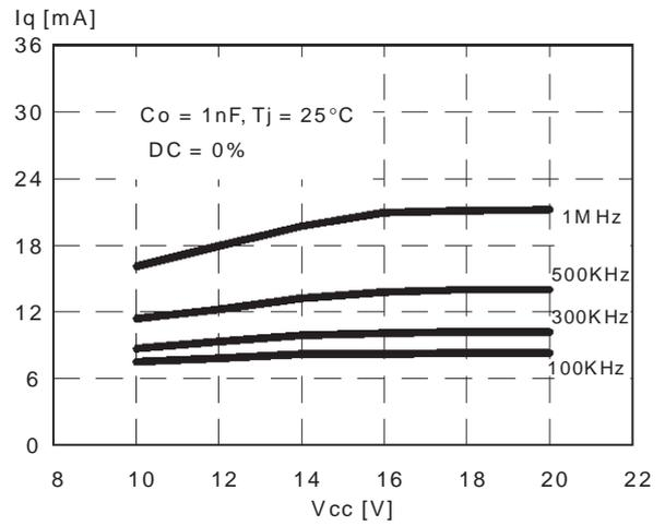
**Figure 5. Quiescent current vs. input voltage and switching frequency.**
