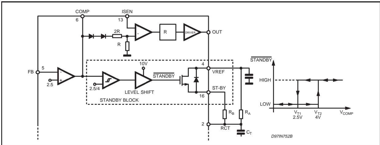
and the output switching frequency will be halved with respect to the oscillator one because an internal T flip-flop (see block diagram) is activated. Fig. 30 shows the operation.
