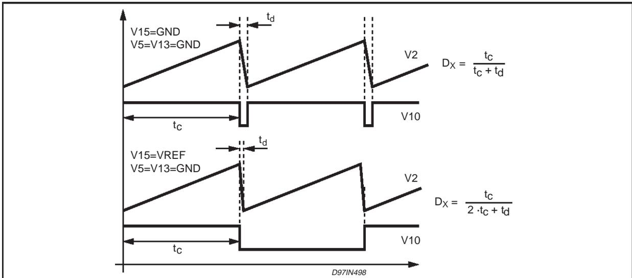
Figure 31. Standby function internal schematic and operation.
