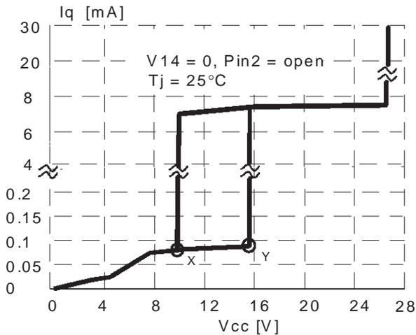
Figure 2. L5991 - Quiescent current vs. input voltage (after disable).
