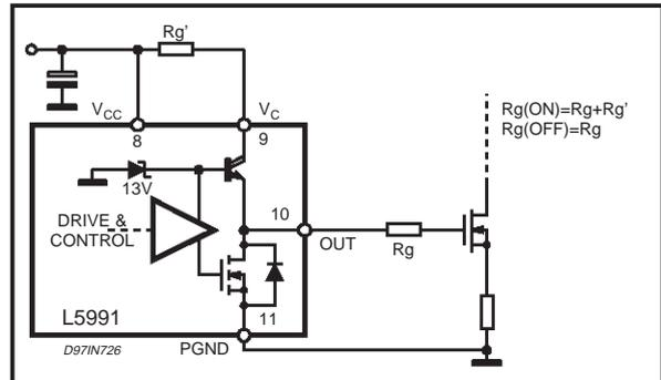
**Pin 10.** OUT (Driver Output). This pin is the output of the driver stage of the external power switch. Usually, this will be a PowerMOS, although the driver is powerful enough to drive BJT's (1.6A source, 2A sink, peak).
