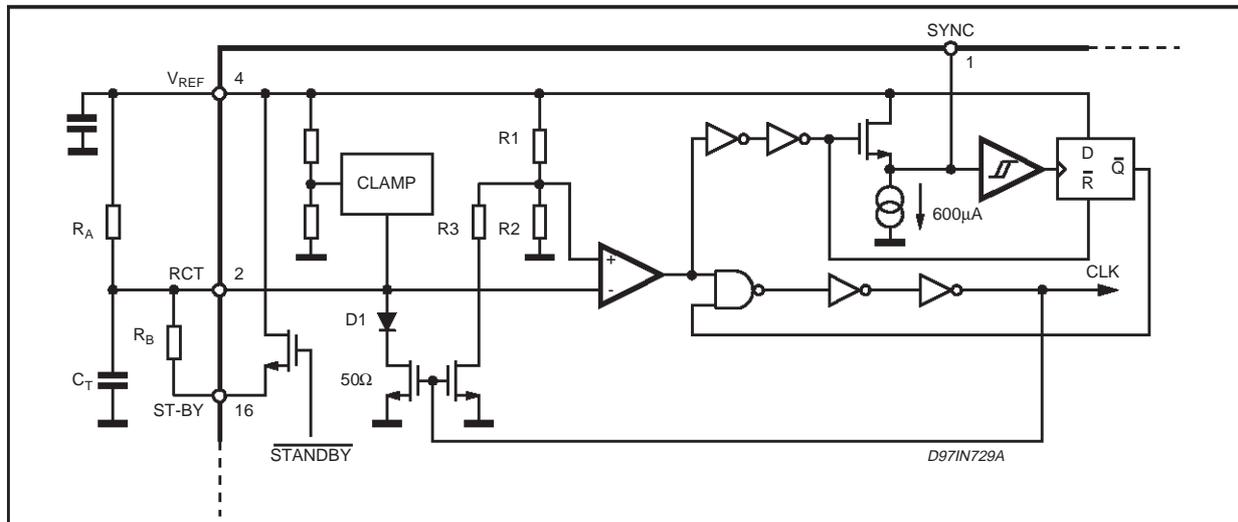
The oscillation frequency can be established with the aid of the diagrams of fig. 13, where  $R_T$  will be intended as the parallel of  $R_A$  and  $R_B$  in normal operation and  $R_T = R_A$  in standby, or considering the following approximate relationships:
