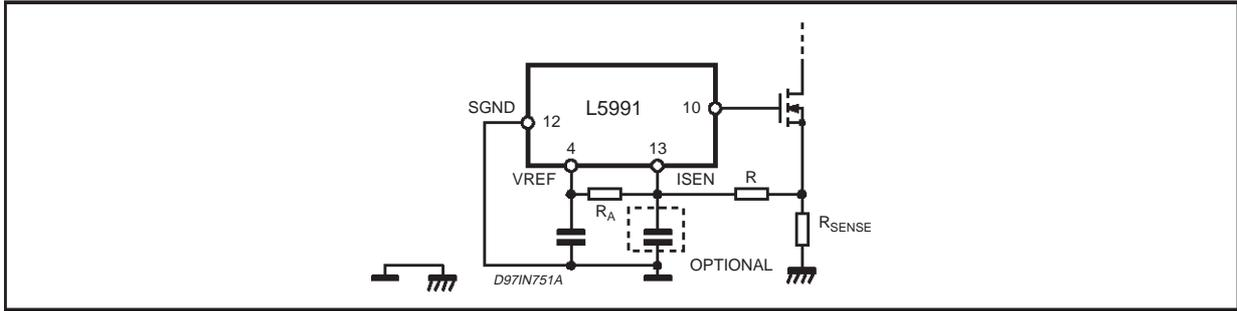
Figure 35. Isolated MOSFET Drive & Current Transformer Sensing in 2-switch Topologies.
