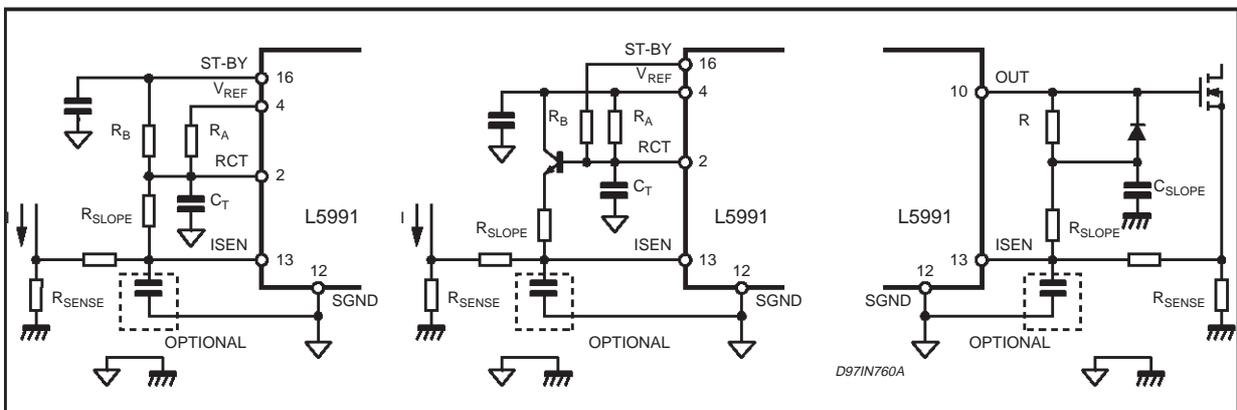
Figure 41. Protection against overvoltage/feedback disconnection (latched)
