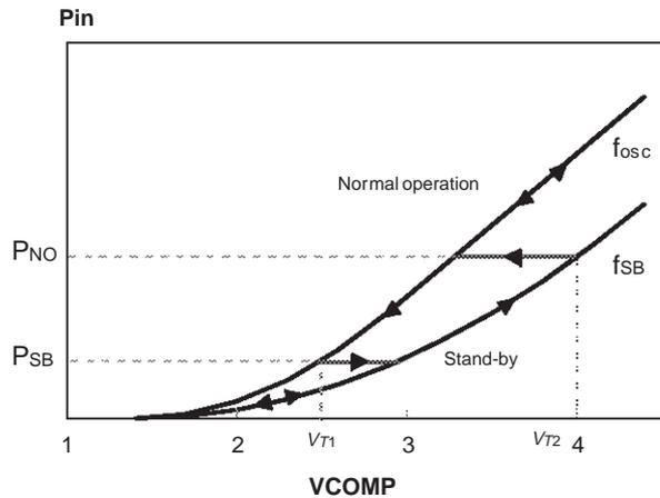
atically the master. During the ramp-up of the oscillator the pin is pulled low by a  $600\mu A$  internal sink current generator. During the falling edge, that is when the pulse is released, the  $600\mu A$  pull-down is disconnected. The pin becomes a generator whose source capability is typically  $7mA$  (with a voltage still higher than  $3.5V$ ).
