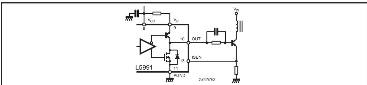
Figure 38. Typical E/A compensation networks.
