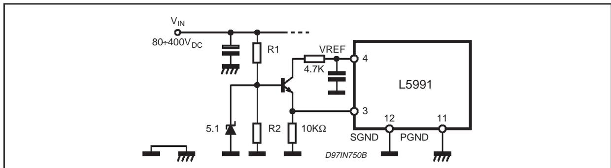
Figure 47. Synchronization to flyback pulses (for monitors).
