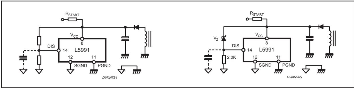
Figure 42 Protection against overvoltage/feedback disconnection (not latched)
