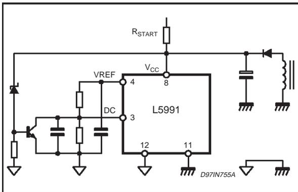
Figure 43. Device shutdown on overcurrent
