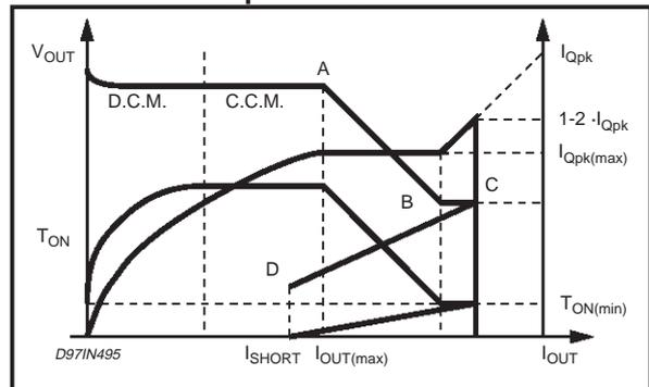
the ON-time of the power switch can be reduced (from A to B). After the minimum ON-time is reached (from B onwards) the current is out of control.
