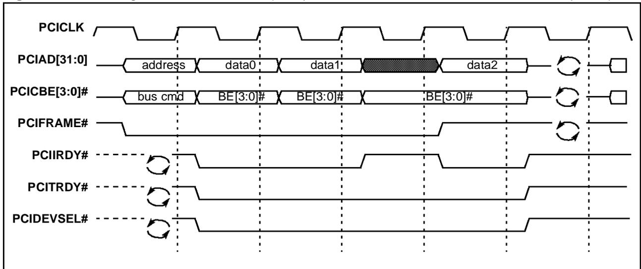
Figure 14. PCI Target read - Slave Read (1-cycle single word read)
