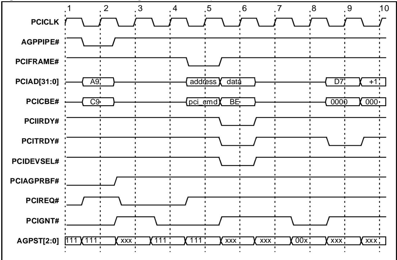
Figure 5. Basic AGP pipeline concept
