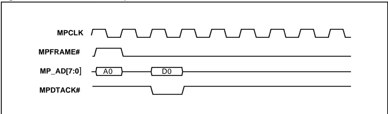
Figure 44. CPU read\_receive cycle - throttled by slave
