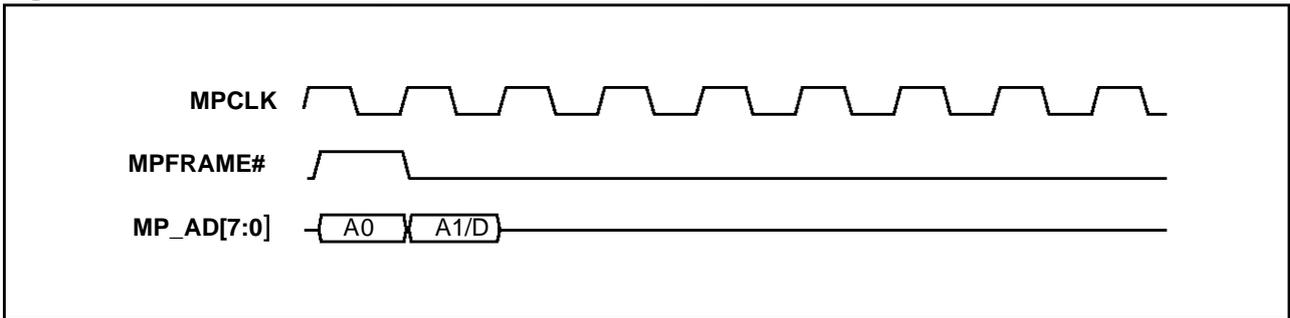
Figure 43. CPU read\_receive cycle
