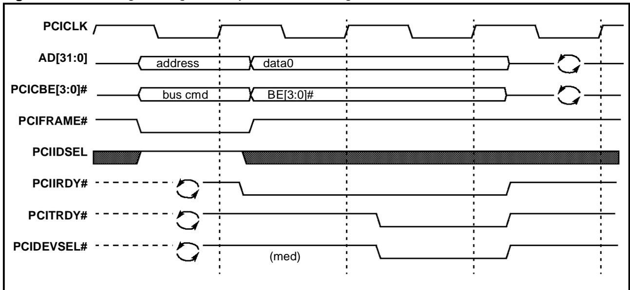
Figure 19. PCI Target configuration cycle - Slave Configuration Read
