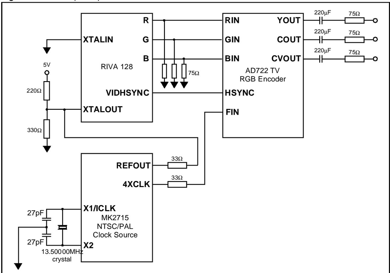
**Figure 60.** Interface to monitor or television
