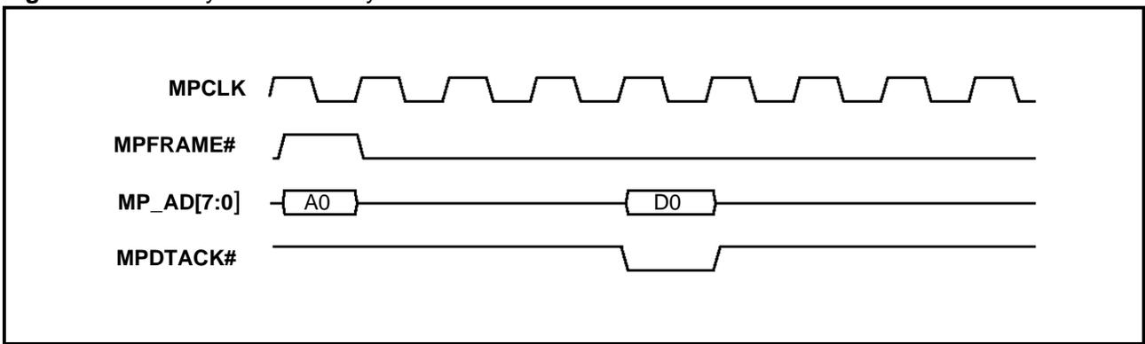
Figure 40. CPU write cycle
