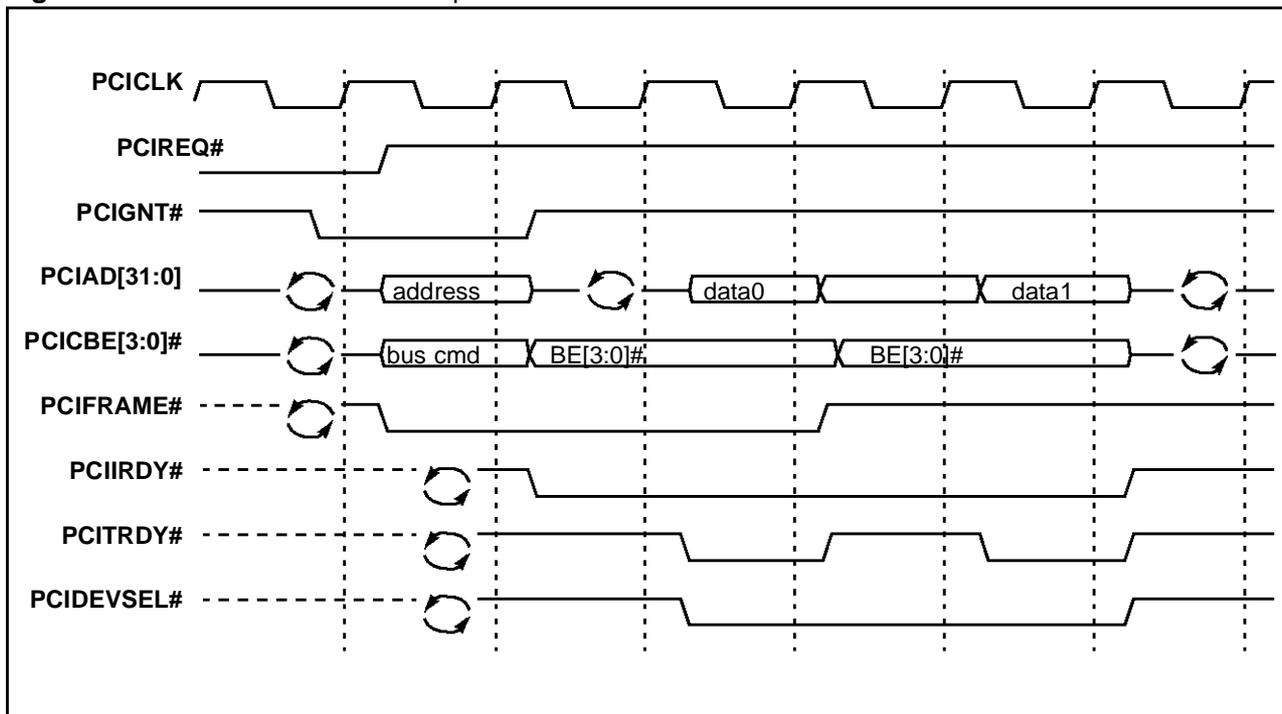
Note: The RIVA 128 does not generate fast back to back cycles as a bus master
