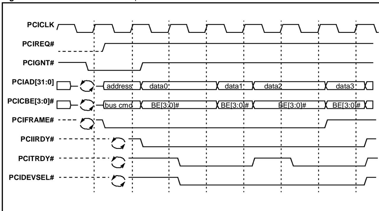
Figure 17. PCI Master read - multiple word
