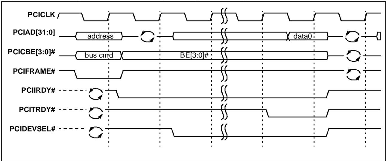
Figure 16. PCI Master write - multiple word
