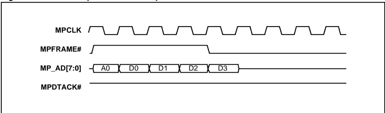
Figure 46. CD write cycle - terminated by slave in middle of transfer
