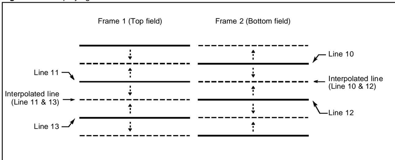
The RIVA 128 video overlay handles interlaced video by displaying every field, at the original frame rate of the video (50Hz for PAL and 60Hz for NTSC). The video scaling logic upscales, in the vertical direction, the luma components in each field and linearly interpolates successive lines to produce the missing lines of each field. This interpolated scale is applied such that the full frame size of each field is stretched to the desired height.
