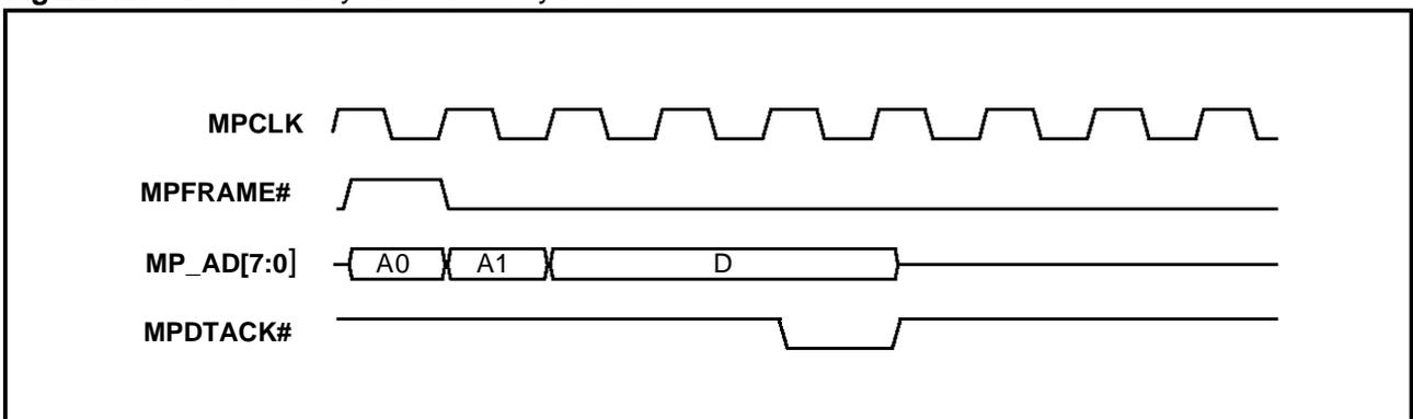
Figure 42. CPU read issue cycle - cannot be throttled by slave
