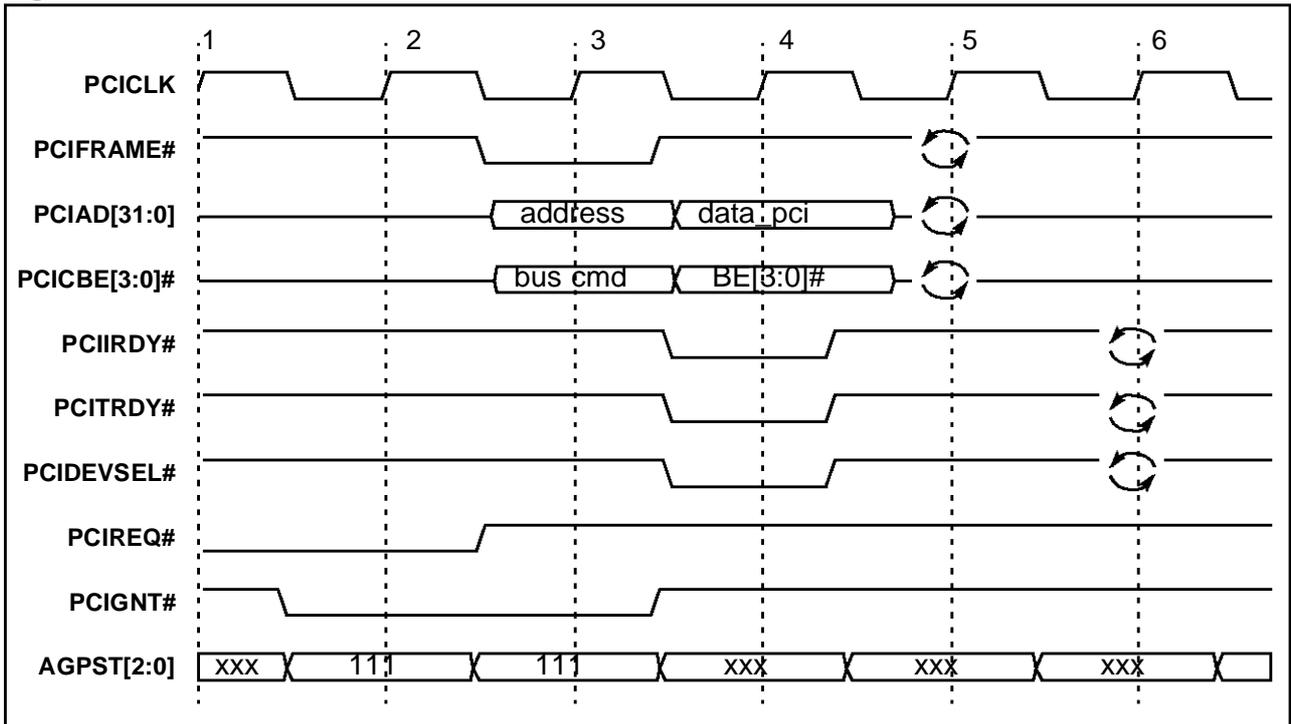
An example of a PCI transaction occurring between an AGP command cycle and return of data is shown in Figure 4. This shows the smallest number of cycles during which an AGP request can be enqueued, a PCI transaction performed and AGP read data returned.
