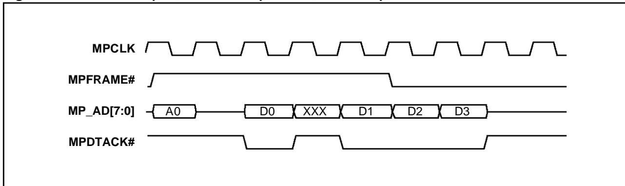
Figure 50. UCD read cycle, terminated by slave, throttled by slave
