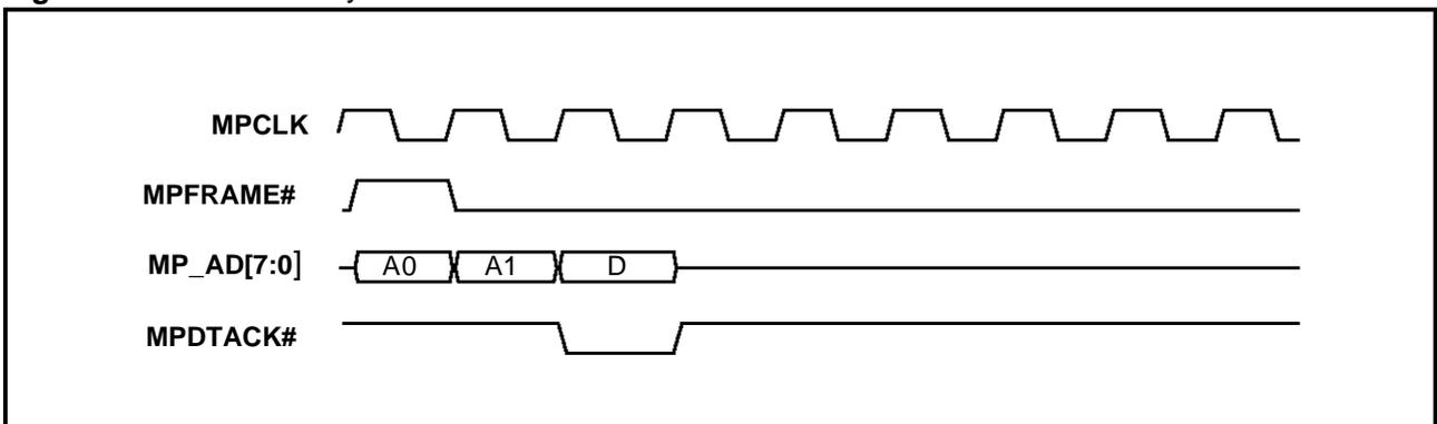
Figure 41. CPU write cycle throttled by slave
