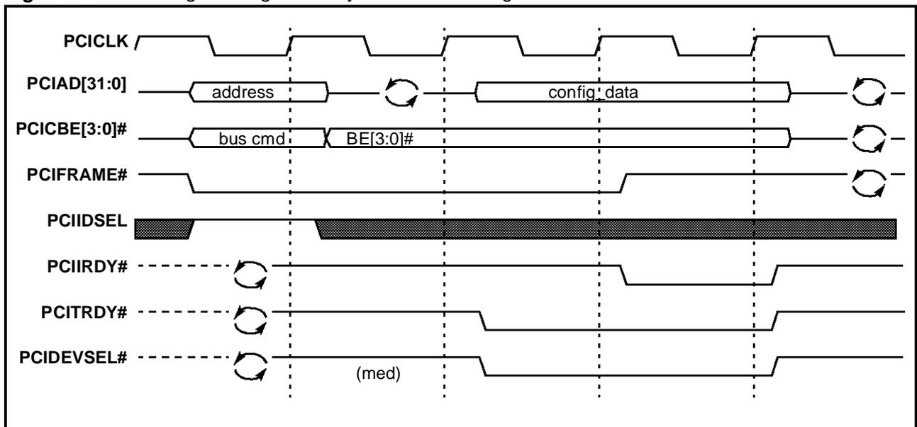
Figure 20. PCI basic arbitration cycle
