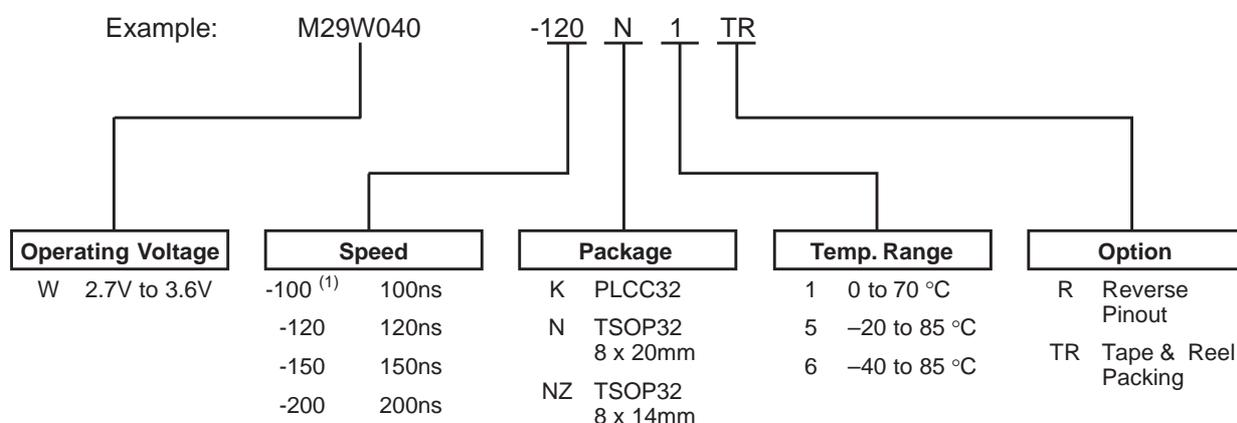
**Note:** 1. This speed is obtained with a supply voltage range of  $V_{CC} = 3.3V \pm 0.3V$  and a load capacitance at 30pF.
