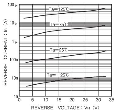
Fig. 2 Reverse characteristics
