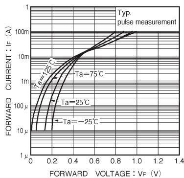
Fig. 1 Forward characteristics
