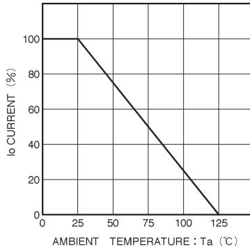
Fig. 5 Derating curve
