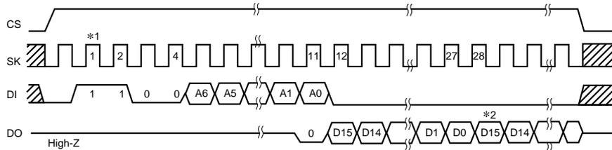
\*1 If the first data input following the rise of the start bit CS is "1", the start bit is acknowledged. Also, if a "1" is input following several zeroes in succession, the "1" is recognized as the start bit, and subsequent operation commences. This applies also to all commands described subsequently.
