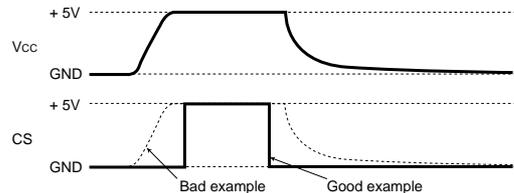
(Bad example) Here, the CS pin is pulled up to  $V_{CC}$ . In this case, CS is HIGH (active state). Please be aware that the EEPROM may perform erroneous operations or write erroneous data because of noise or other factors. This can occur even if the CS input is high-Z.
