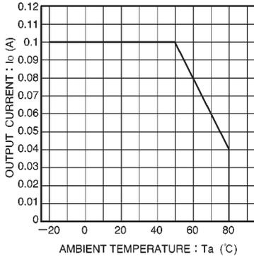
Fig.7 Derating curve
