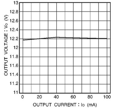
Fig.9 Output characteristic
