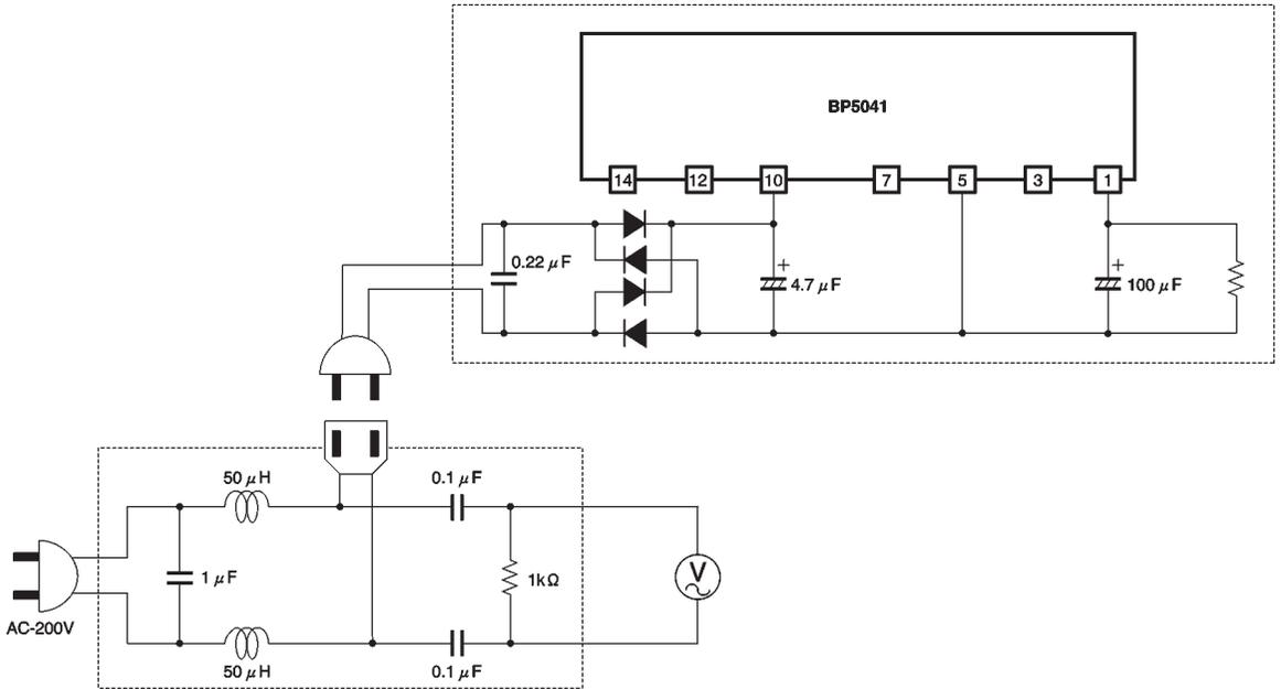
Fig.6 Test circuit
