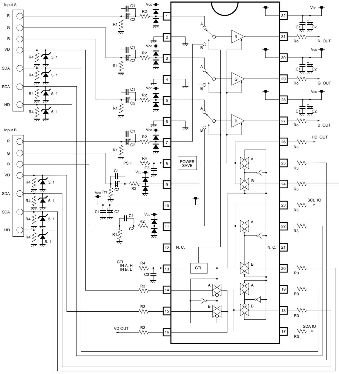
Note: The Ro value differs depending on the load capacitance.
