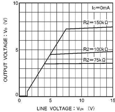
Fig. 6 Output voltage vs. line voltage (with R2)
