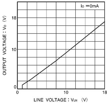
Fig. 5 Output voltage vs. line voltage (without R2)
