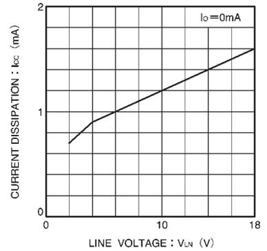
Fig. 7 Current dissipation vs. line voltage
