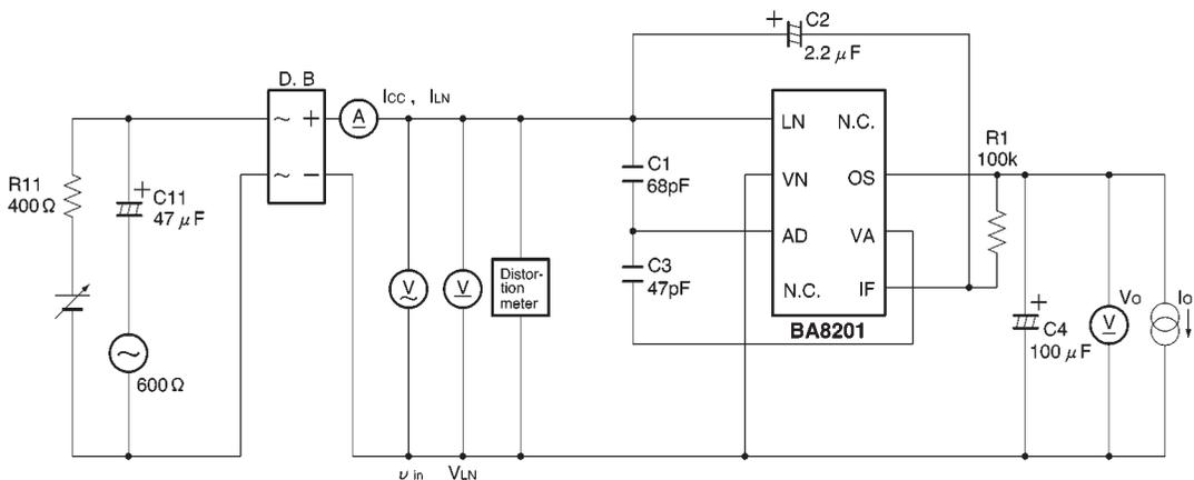
Fig. 1 Measurement circuit (1)
