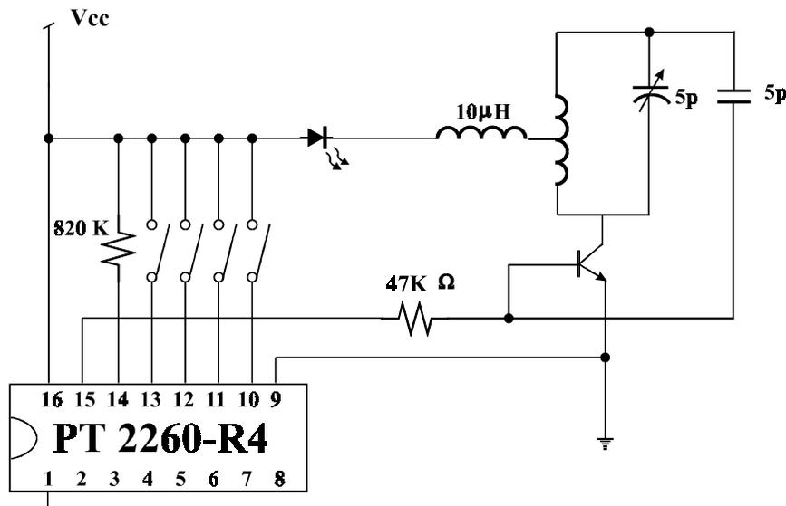
UHF Band 4-Data Transmitter Circuit is recommended.
