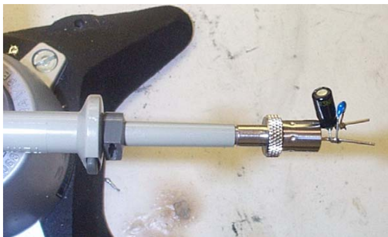
Figure 6 - Oscilloscope Probe with Probe Master 5125BA BNC Adapte
