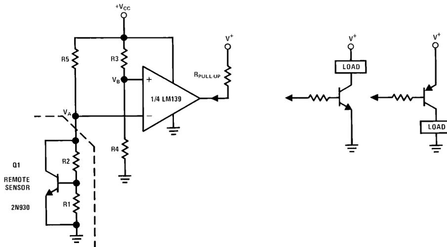
FIGURE 35. Temperature Alarm
