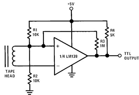
FIGURE 38. Magnetic Tape Reader with TTL Output
