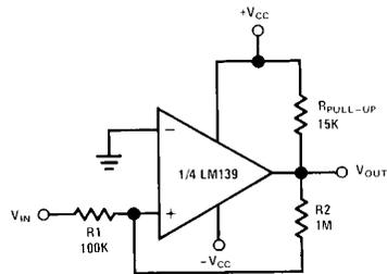
FIGURE 32. Zero Crossing Detector Using Dual Supplies
