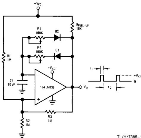
FIGURE 14. Pulse Generator with Variable Duty Cycle
