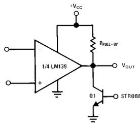
FIGURE 21. Output Strobing Using a Discrete Transistor
