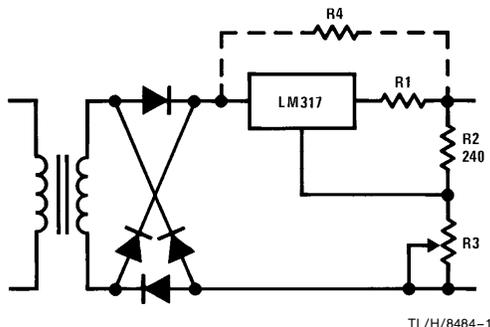
FIGURE 1. Constant Voltage Charging Circuit
