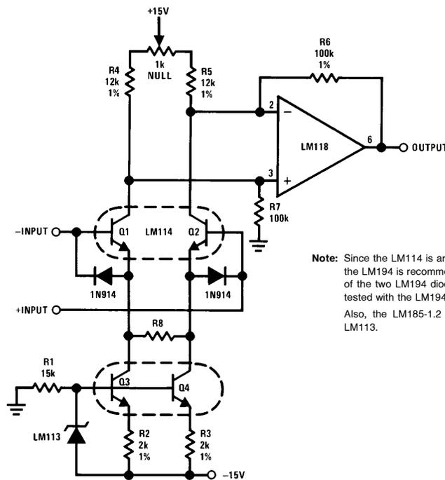
**Note:** Since the LM114 is an obsolete part, substitution of the LM194 is recommended, along with the removal of the two LM194 diodes. This circuit has not been tested with the LM194 included.
