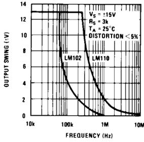
Power bandwidth of the LM110 is five times larger than the LM102.
