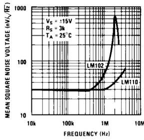
Eliminating zeners reduces typical high frequency noise by nearly a factor of 10. Worst case noise is reduced even more. High frequency noise of LM102 has caused problems when it was included inside feedback loop with other IC op amps.
