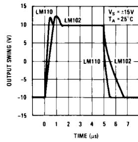
Large signal pulse response shows  $40V/\mu s$  slew for LM110 and  $10V/\mu s$  for LM102. Leading edge overshoot on LM110 is virtually eliminated, so external clamp diode frequently required on the LM102 is not needed.
