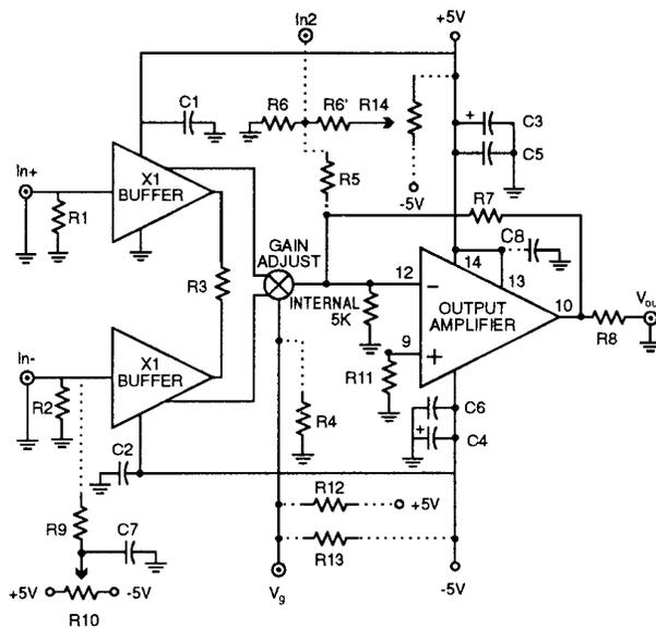
**Figure 1: External components & amplifier internal block diagram**
