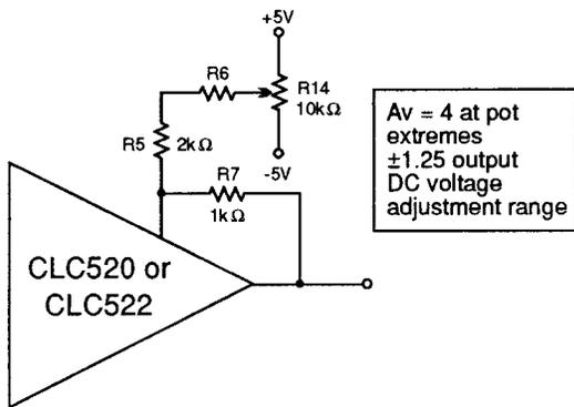
**Figure 6: Summing in an output DC offset**
