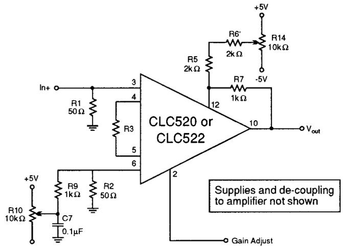
**Figure 7: Input and output stage DC nulling**
