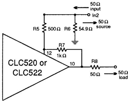
**Figure 5: Summing a high-speed signal into the output**
