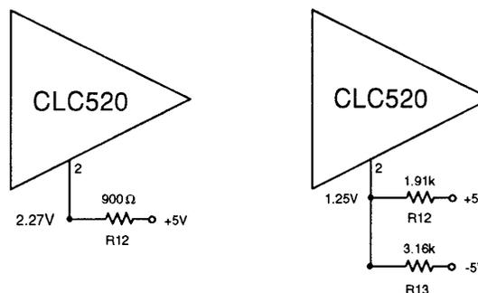
Figure 4: Setting up for the fixed maximum gain
