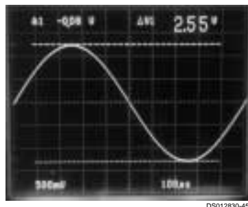
FIGURE 2. Output Swing Performance of the LMC6035 per the Circuit of Figure 1
