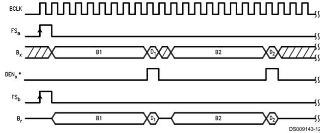
\*Note: In TES mode, DEN<sub>x</sub> outputs SCLK synchronized to the S interface. Format 1, SCLK = 2.048 MHz, Format 2, SCLK = 256 kHz, Format 3, SCLK = 512 kHz, Format 4, SCLK = 2.56 MHz.
