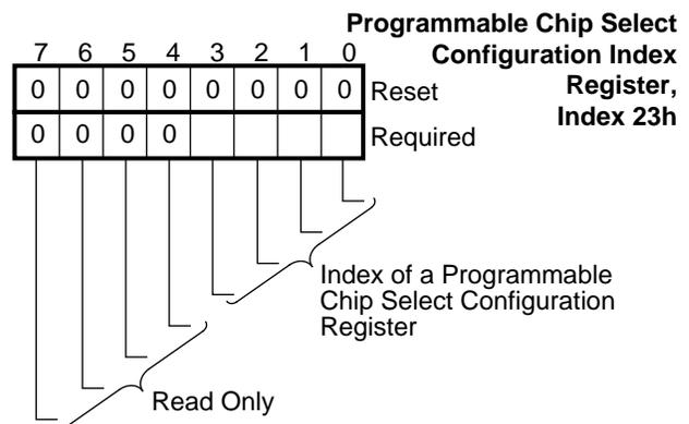
**FIGURE 2-5. Programmable Chip Select Configuration Index Register Bitmap**
