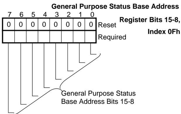
**FIGURE 10-18. General Purpose Base Address Bits 15-8 Register Bitmap**
