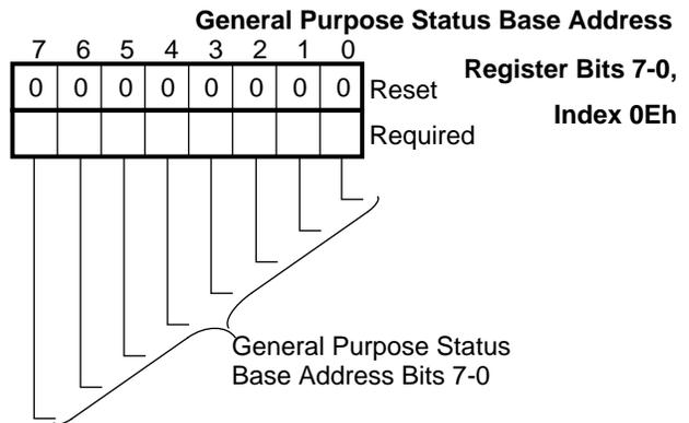
**FIGURE 10-17. General Purpose Base Address Bits 7-0 Register Bitmap**
