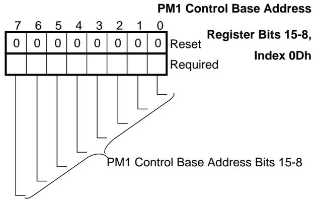
**FIGURE 10-16. PM1 Control Base Address Bits 15-8 Register Bitmap**
