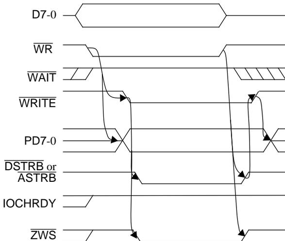
**FIGURE 6-14. EPP Write with Zero Wait States**
