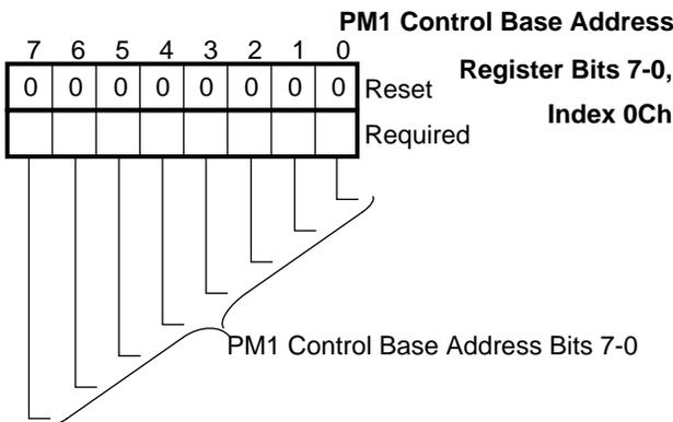
**FIGURE 10-15. PM1 Control Base Address Bits 7-0 Register Bitmap**
