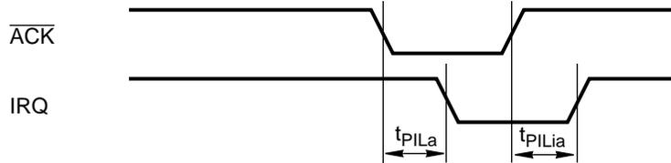
FIGURE 14-21. Parallel Port Interrupt Timing (Compatible Mode)
