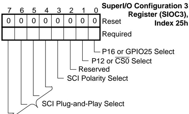
**FIGURE 2-7. SIOC3 Register Bitmap**
