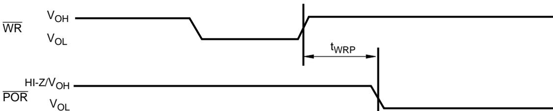
FIGURE 14-36. SMI\_CMD/PM1\_CNT\_LOW/PM1\_CNT\_HIGH Register Write to  $\overline{POR}$  Timing
