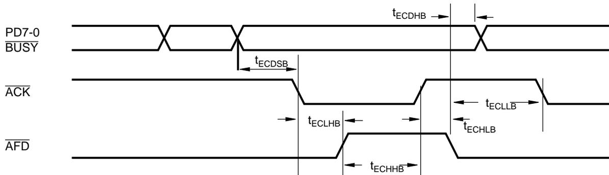
FIGURE 14-27. ECP Parallel Port Backward Timing Diagram
