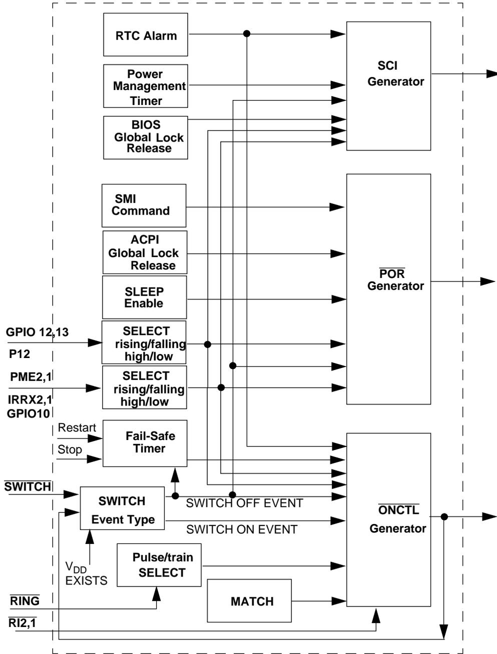
FIGURE 4-12.  $\overline{\text{POR}}$ , SCI and  $\overline{\text{ONCTL}}$  Generation
