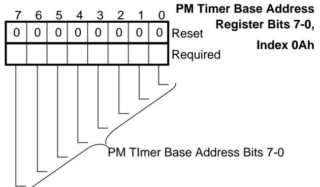
**FIGURE 10-13. PM Timer Base Address Bits 7-0 Register Bitmap**
