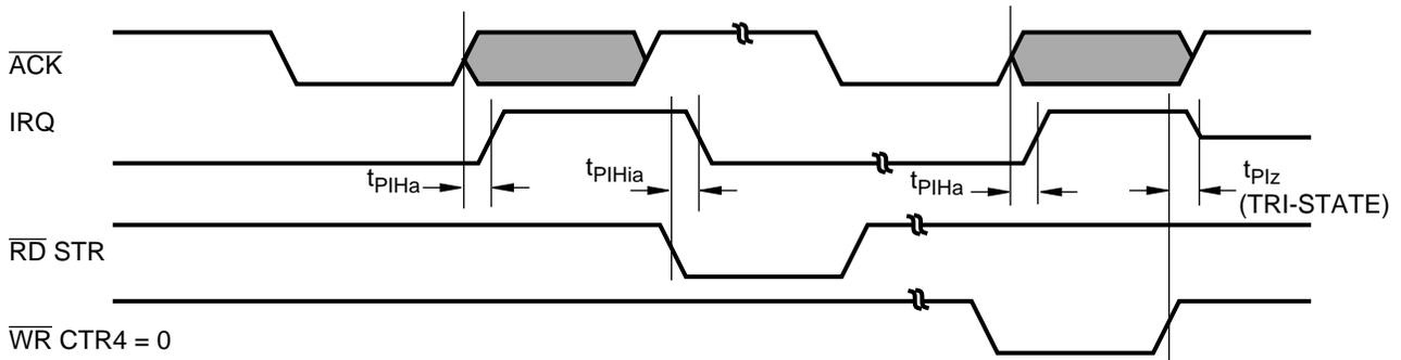
FIGURE 14-22. Parallel Port Interrupt Timing (Extended Mode)
