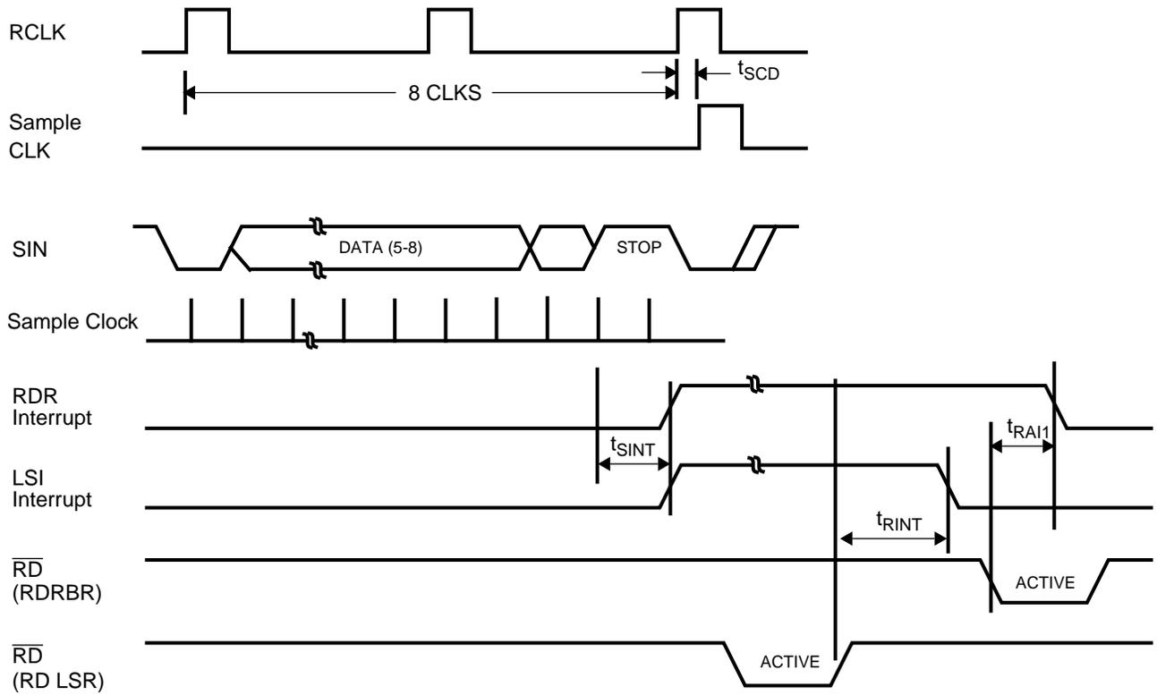
FIGURE 14-8. Receiver Timing
