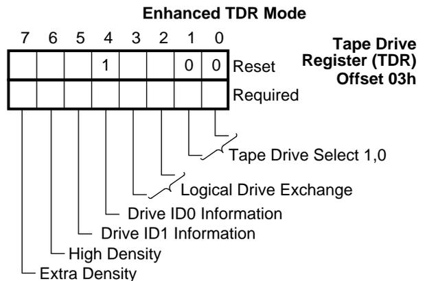
**FIGURE 5-8. TDR Register Bitmap, Enhanced TDR Mode**
