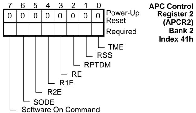
FIGURE 4-15. APCR2 Register Bitmap
