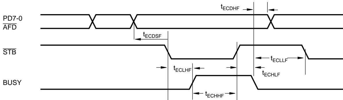
FIGURE 14-26. ECP Parallel Port Forward Timing Diagram
