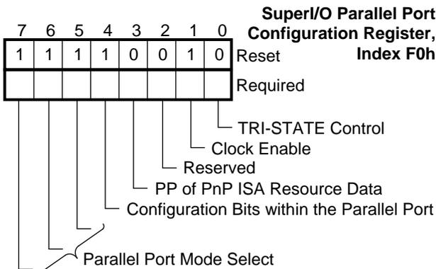
**FIGURE 2-12. Super/I/O Parallel Port Configuration Register Bitmap**
