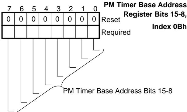
**FIGURE 10-14. PM Timer Base Address Bits 15-8 Register Bitmap**
