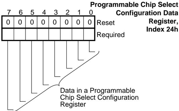
**FIGURE 2-6. Programmable Chip Select Configuration Data Register Bitmap**
