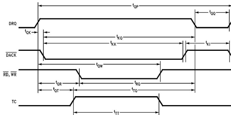
FIGURE 9-8. DMA Timing
