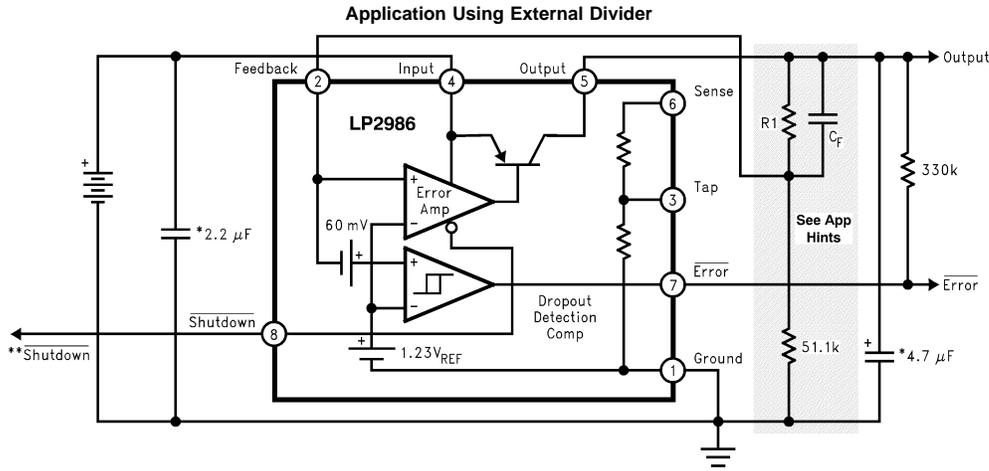
\* Minimum capacitance shown to assure stability, but may be increased without limit. Larger output capacitor provides improved dynamic response.
