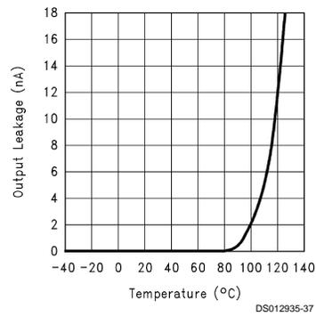
**Typical Performance Characteristics** Unless otherwise specified:  $T_A = 25^\circ\text{C}$ ,  $C_{OUT} = 4.7\ \mu\text{F}$ ,  $C_{IN} = 2.2\ \mu\text{F}$ , S/D is tied to  $V_{IN}$ ,  $V_{IN} = V_O(\text{NOM}) + 1\text{V}$ ,  $I_L = 1\ \text{mA}$ . (Continued)
