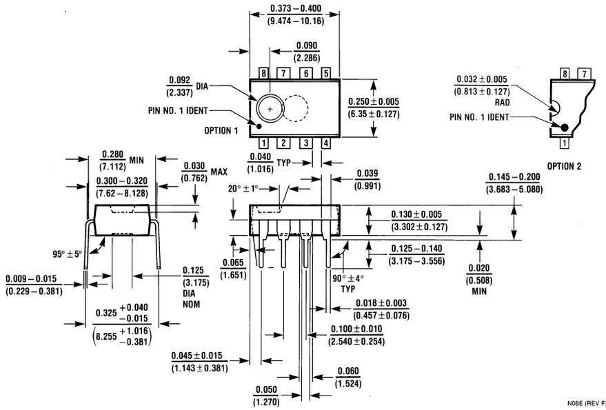
**8-Pin Molded Dual-In-Line Package**
