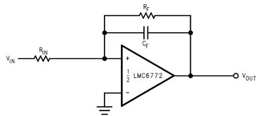
**FIGURE 3. Canceling the Effect of Input Capacitance**
