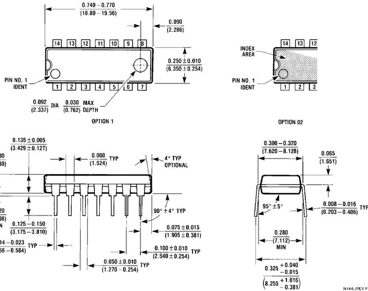
**14-Lead Molded Dual-In-Line Package**
