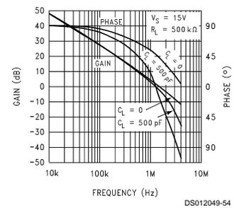
**Typical Performance Characteristics**  $V_S = +15V$ , Single Supply,  $T_A = 25^\circ C$  unless otherwise specified (Continued)
