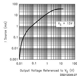
**Typical Performance Characteristics**  $V_S = +15V$ , Single Supply,  $T_A = 25^\circ C$  unless otherwise specified (Continued)
