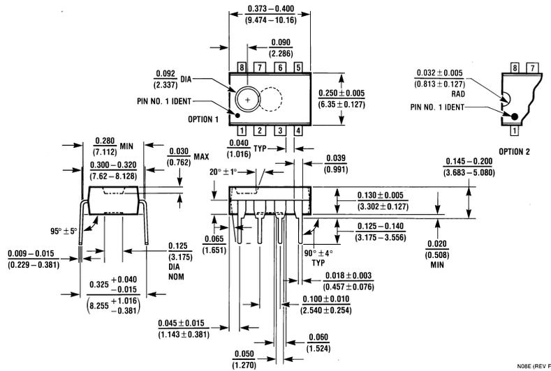
**8-Lead (0.300" Wide) Molded Dual-In-Line Package**
