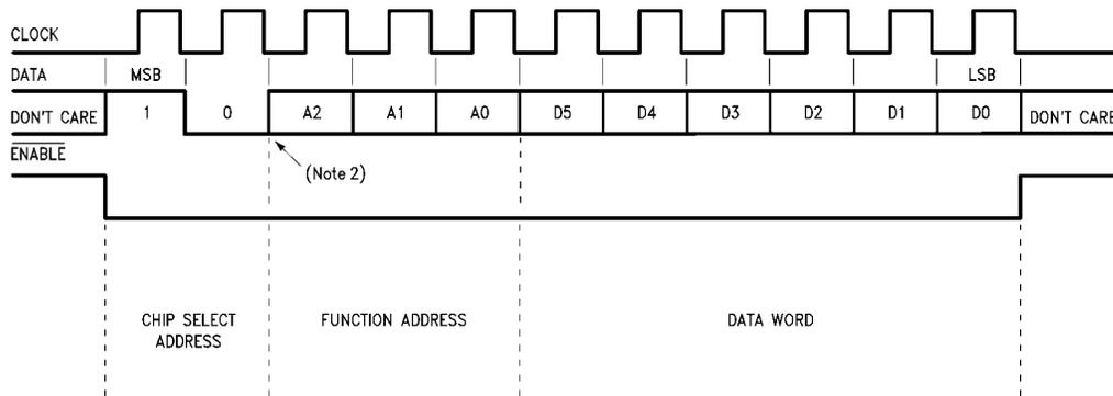
**Note 1:** Negative transition on  $\overline{\text{ENABLE}}$  clears previous address. Clock must be low during transition.
