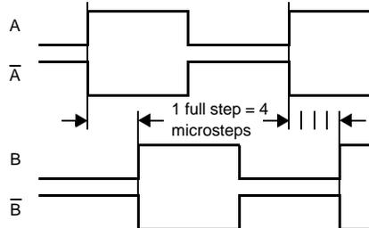
Figure 16: Stepper Motor Waveform - Full Stepping
