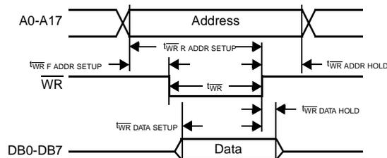
Figure 8: SRAM Write
