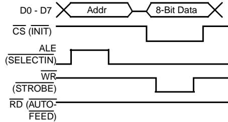
**Figure 56: Writing to the Configuration Register ( $\mu\text{P}$ )**
