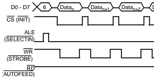
**Figure 58: Writing to the Configuration Register ( $\mu\text{P}$ )**
