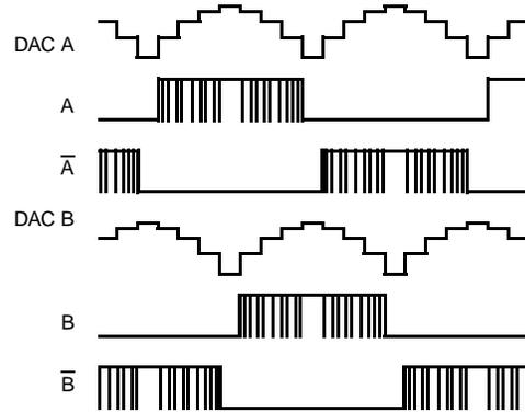
Figure 19: Stepper Motor Waveform - LM9830 Signals
