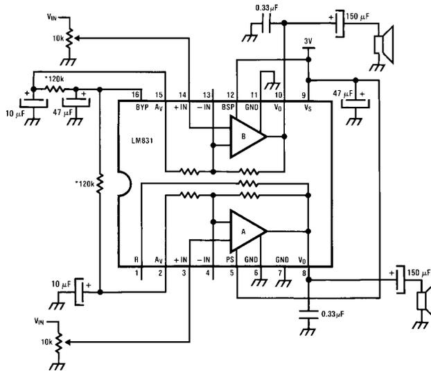
$P_{OUT} = 150$  mW/Ch, BW = 300 Hz to 35 kHz
