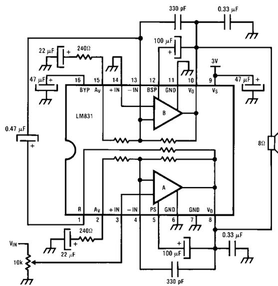
$A_V = 40 \text{ dB}$ ,  $BW = 20 \text{ Hz to } 20 \text{ kHz}$
