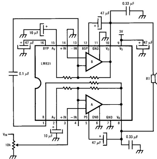
$A_V = 52 \text{ dB}$ ,  $BW = 250 \text{ Hz to } 25 \text{ kHz}$
