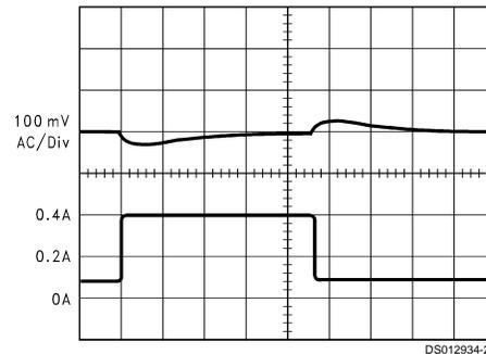
A: Output Voltage, 100 mV/div, AC-Coupled
