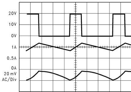
A:  $V_{SW}$  Pin Voltage, 10 V/div.
