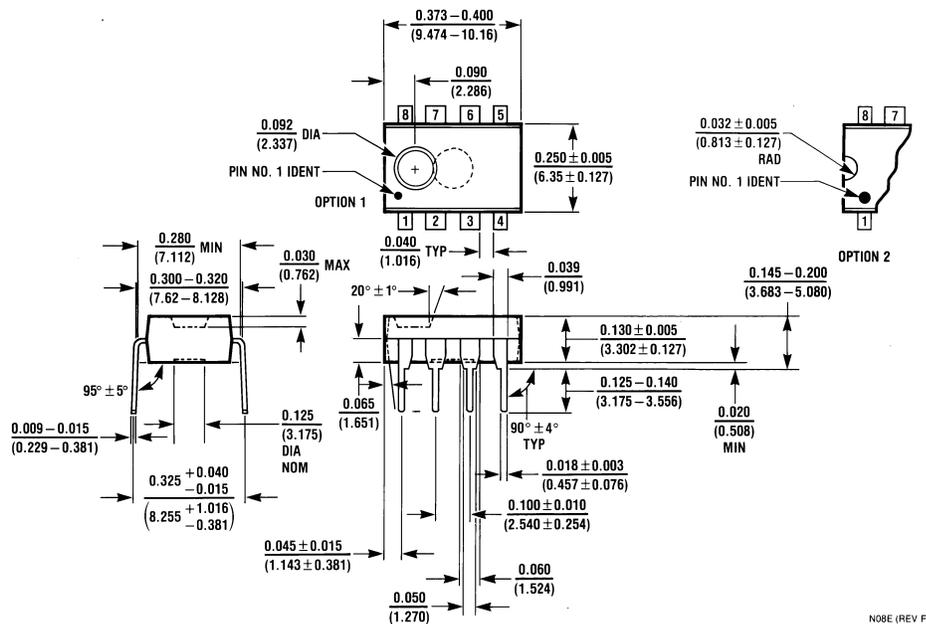
**8-Lead (0.300" Wide) Molded Dual-In-Line Package**
