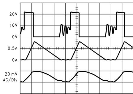
A:  $V_{SW}$  Pin Voltage, 10 V/div.
