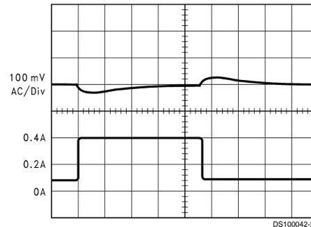
A: Output Voltage, 100 mV/div, AC-Coupled
