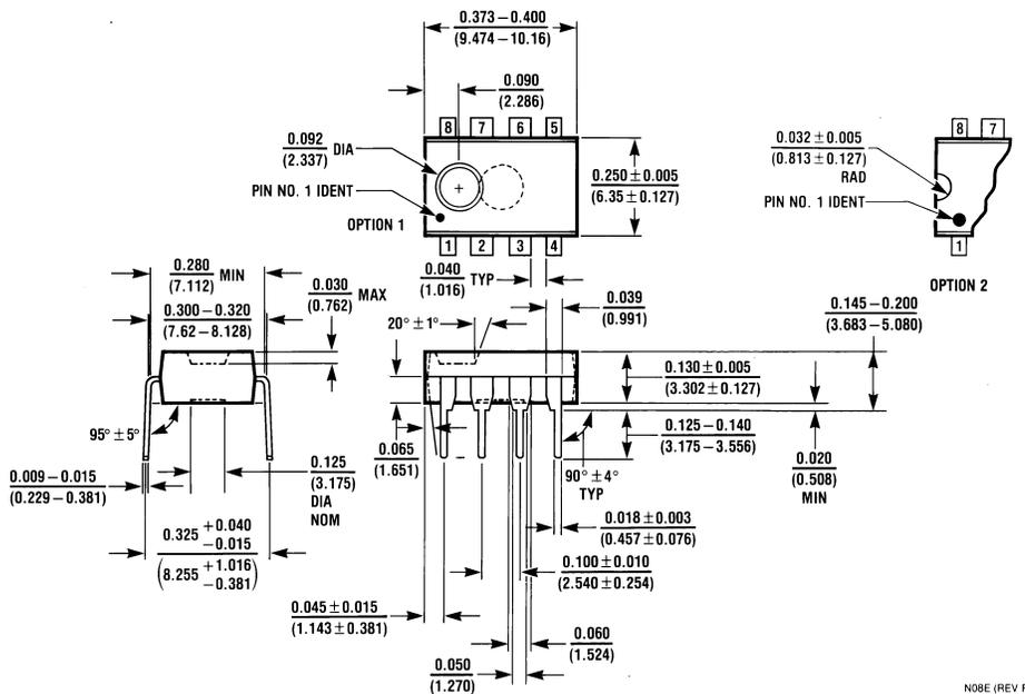
**8-Lead (0.300" Wide) Molded Dual-In-Line Package**
