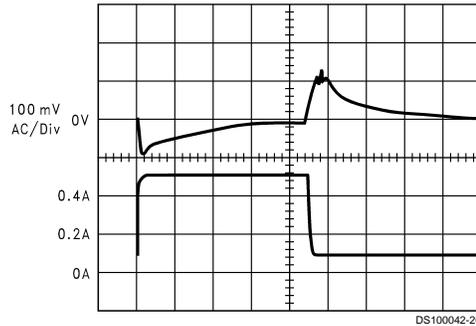
A: Output Voltage, 100 mV/div, AC-Coupled
