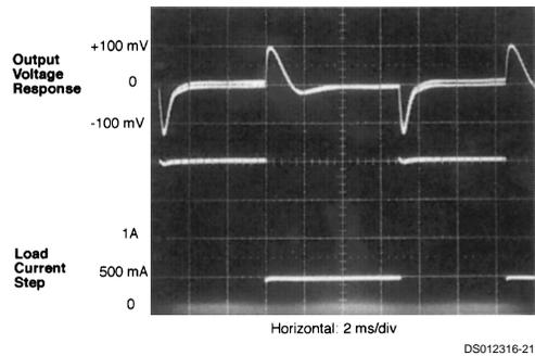
FIGURE 35.  $V_{OUT}$  Response to Load Current Step
