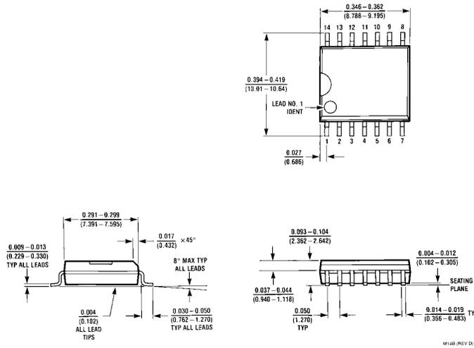
**Molded SOIC Package (M)**
