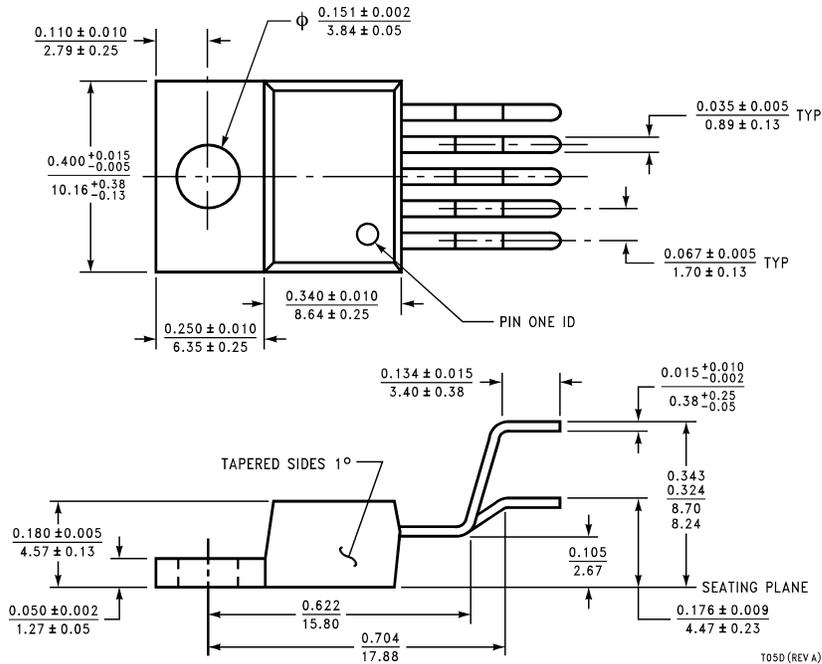
**Bent, Staggered 5-Lead TO-220 (T)**
